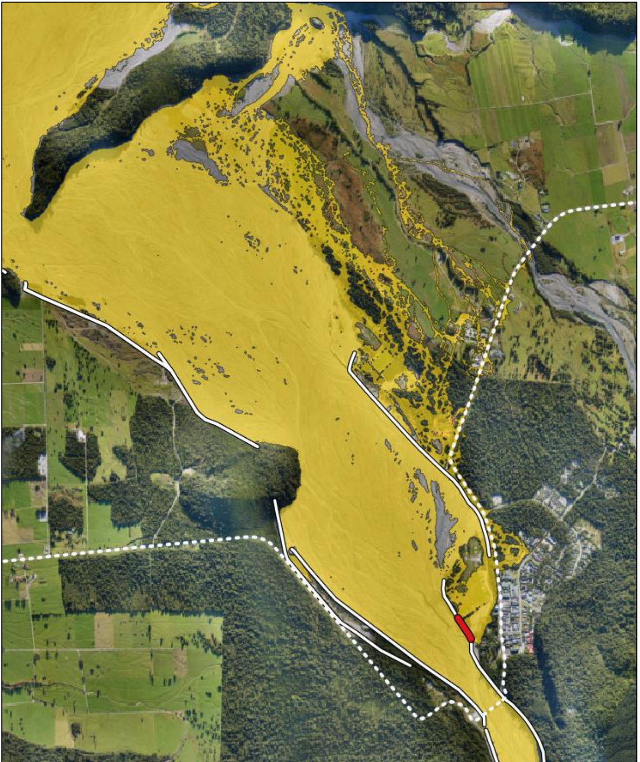
Figure 14-8 - Example of a 2,500 m 3 /s flood extent from a breach of the Heliport stopbank from the LRS fixed bed 2D hydraulic model. The protection network is shown with the white lines, and SH6 by the dashed white line.
