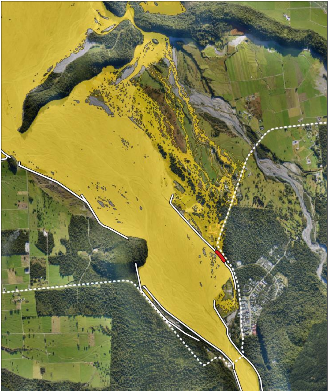
Figure 14-10 - Example of a 2,500 \text{ m}^3/\text{s} flood extent from a breach of the 55kph corner NZTA stopbank, at the corner itself from the LRS fixed bed 2D hydraulic model. The protection network is shown with the white lines, and SH6 by the dashed white line.
